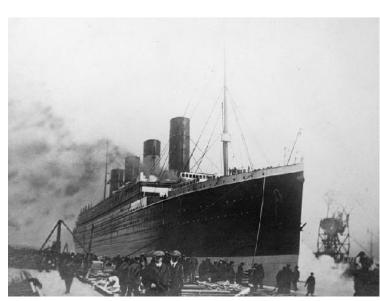
Because the Titanic's compartments were not capped at the top, water from the ruptured compartments filled each succeeding compartment, causing the bow to sink and the stern to be raised up to an almost vertical position above the water. Then the Titanic broke in half, and, at about 2:20 a.m. on April 15, stern and bow sank to the ocean floor.
